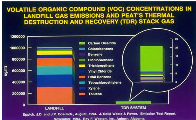
Comparison of Landfill Emissions vs. Plasma Pyrolysis
