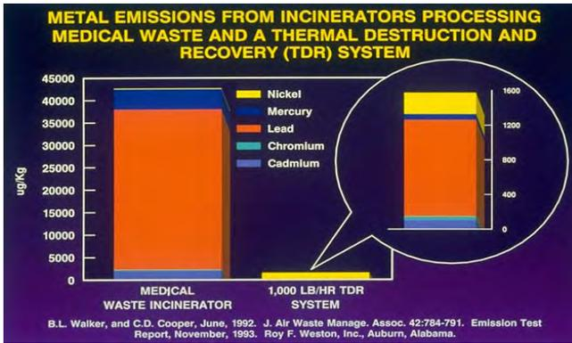
Comparison of Emissions—Incineration vs. Plasma Pyrolysis
