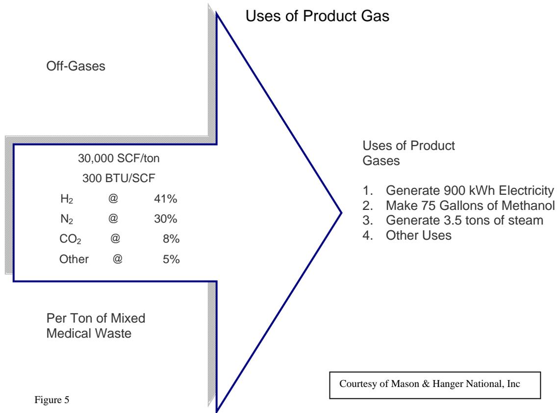
encapsulates cadmium, lead, mercury, chromium and TACs. The vitrified solid from the plasma torch contains the balance of the waste products that did not change into gas. These will not release heavy metals or pollution to the environment. Permissible concentrations of the EP Toxicity test are listed below. Each ton of medical waste processed will produce 100 pounds of slag.
